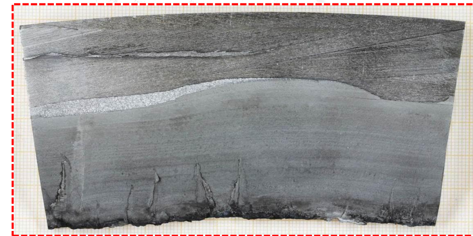
Cleaned fracture surface
